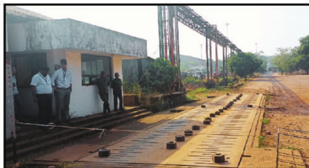
Department conducted inspection of Road weigh bridge at an Industrial Unit for erratic weight measurement.
